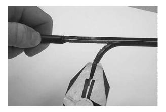
Figure 4 – Peel off the cable jacket.
