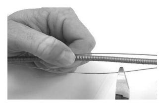
Figure 5 – Measure and cut the strength members.
