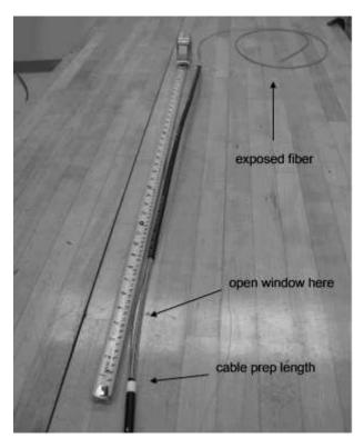
Figure 14 – Cut a window in jacket to expose the buffer tube.
