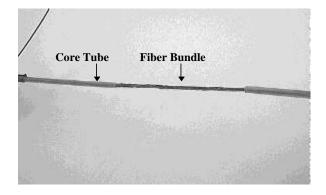
Figure 9 – Remove the buffer tube and cable jacket to expose the fiber bundle.
