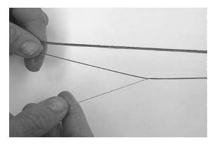
Figure 10 - Separate the fiber bundles.
